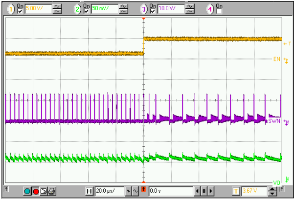
Top to Bottom: SWN_Slave, SWM, V O Figure 11. On Line Mode Change (CCM → DCM)
