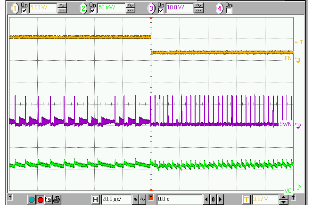
Top to Bottom: EN, SWM, V O Figure 12. On Line Mode Change (DCM → CCM)
